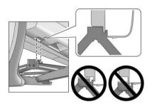
The triangle is located near each wheel on the vehicle's exterior.
